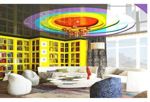
Sitting Room or entrance room concept with coloured PVC fabric seem jointed and in different levels. Any type of light fittings or aperture can be accommodated within the stretch membrane. Being humidity resistant ideal for Kitchen, washroom and above swimming pool.
